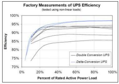
This graph shows the efficiency of a UPS based on the load. A UPS loaded at 60% operates more efficiently than the same UPS loaded to only 20%. The same holds true for CRAC units, server power supplies, and so on.
